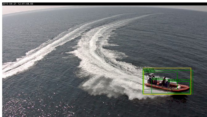
Fig. 12. Multiple detections and scores and one ground truth frame for maritime boat object. Lowering IoU requirement from consumer data setup allows for better evaluation for the system.
